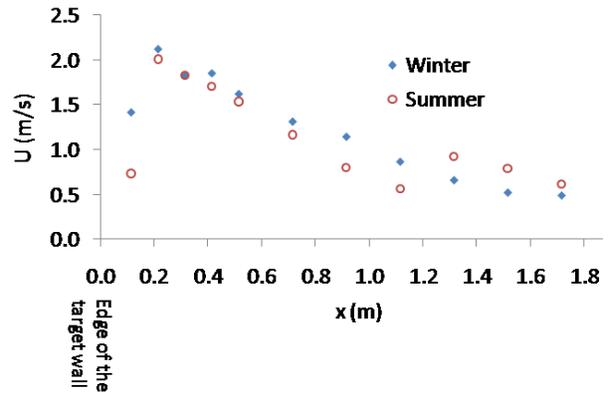
Figure 6. Decay of  $x$  velocity component in  $x$  direction at height 0.8 m from the floor.
