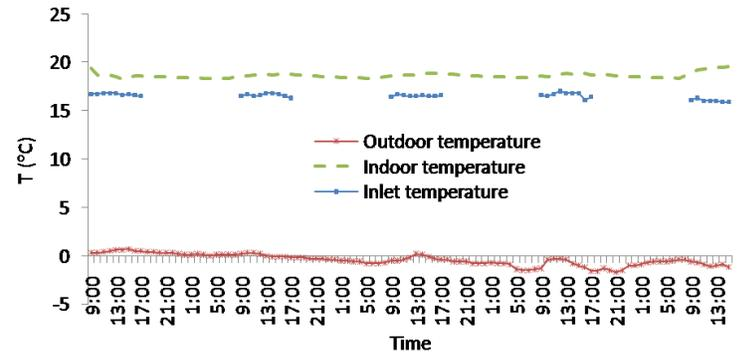
Figure 7b. Measured outdoor, indoor and inlet temperature, winter case.
