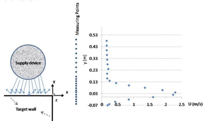
Figure 4. Profile of x velocity component in y direction, winter case.
