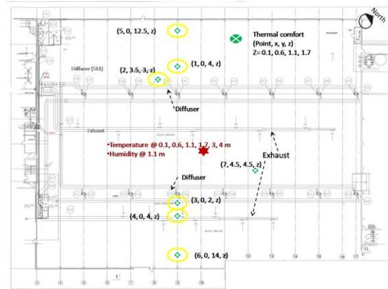
Figure 2. Geometry and position of the measuring points.
