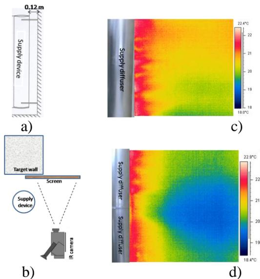
Figure 3. IR image visualization - supply air temperature about  $22 \text{ }^\circ\text{C}$ , air-flow rate  $0.25 \text{ m}^3/\text{s}$ , winter case a) side view b) top view set up c) one supply device d) two supply devices.
